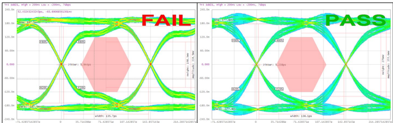
Figure 14: Eye diagram with the WE-CNSW filter (left) and the WE-CNSW HF filter (right) at 7 GBit/s
